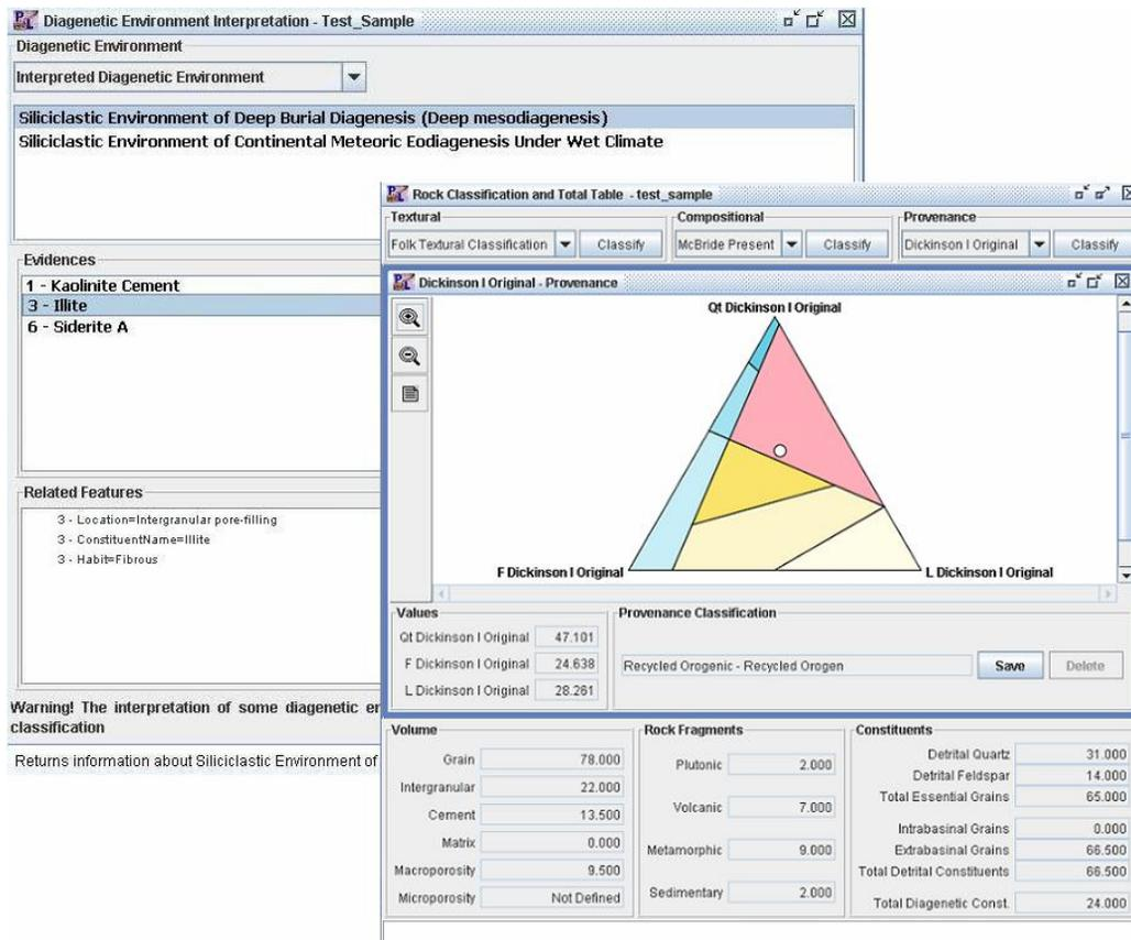
Figure 3: Interface of the Interpretation Module, showing at left a diagenetic environment interpretation, with the corresponding criteria, and at right a provenance detrital mode interpretation (cf. Dickinson, 1985) of a sandstone sample.
