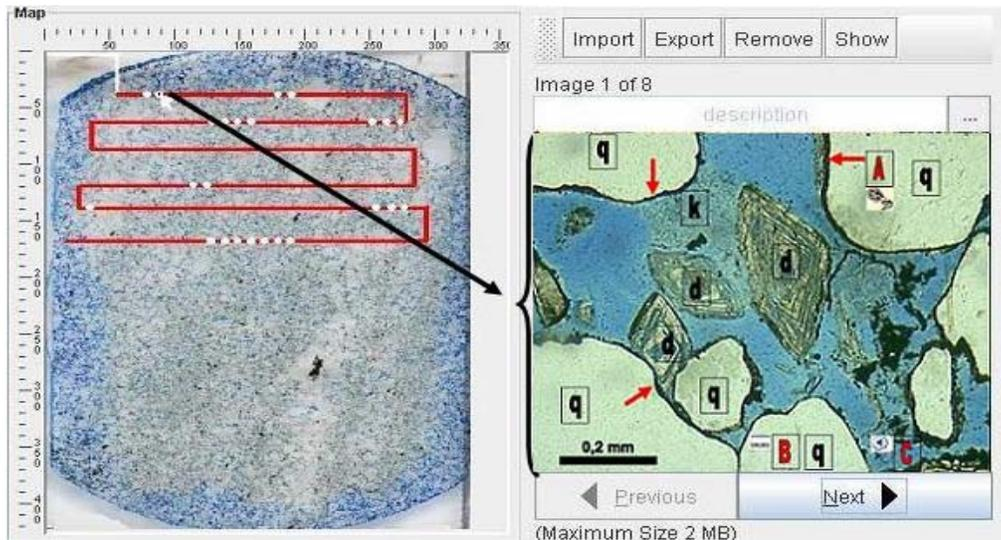
Figure 2: Interface of the Image Annotation Module, which allows the association of features in the photomicrographs to textual comments, WEB links or voice recording files, keeping precise spatial referencing of each image. A map of the analytical pathway and points is shown over a scanned image of the thin-section (left).
