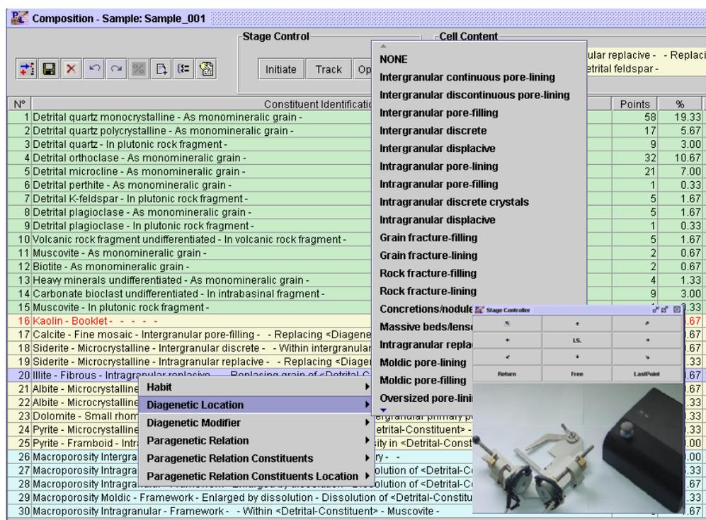
Figure 1: Example of the Compositional Quantification interface from the description of a sandstone sample. Constituents, habits, locations, modifications and paragenetic relations are selected with the mouse, and then points can be counted for each line of description. Inset illustrates the Stageledge® electromechanical microscope stage and its controls.
