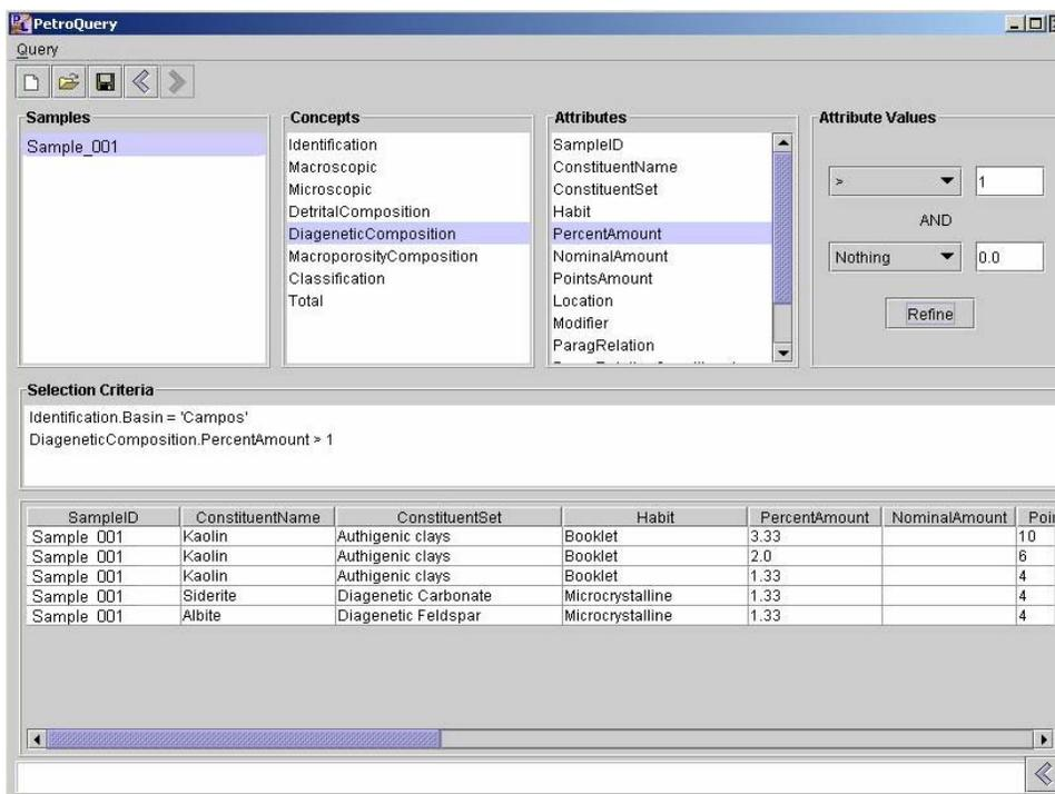
Figure 5: PetroQuery interface illustrating a simulated consultation for the identification of samples with more than 1 % of diagenetic kaolinite in Campos Basin.
